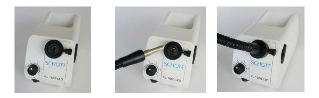
First loosen the locking screw (3) on the light guide socket (4) by turning it anti-clockwise. Insert the light guide as far as the stop and tighten the locking screw (3) by turning it clockwise.
