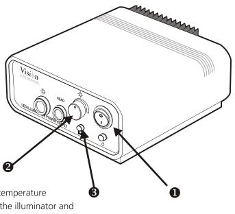
If the temperature protection indicator illuminates, the power to the LED's will gradually reduce until the temperature stabilises. If the indicator remains illuminated, remove the illuminator and ensure neither the air inlet around the objective, nor the fan outlet are obstructed.
