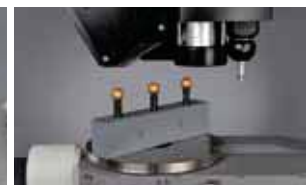
Non-contact measurement precision verification using a ball bar
