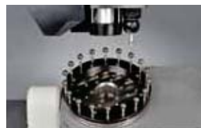
Five-axis precision calibration using a multi-datum ball
