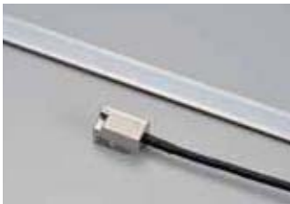
The low thermal expansion linear encoder scales, which are key components in high-precision measurement, are manufactured in-house, using Nikon optical technology.
