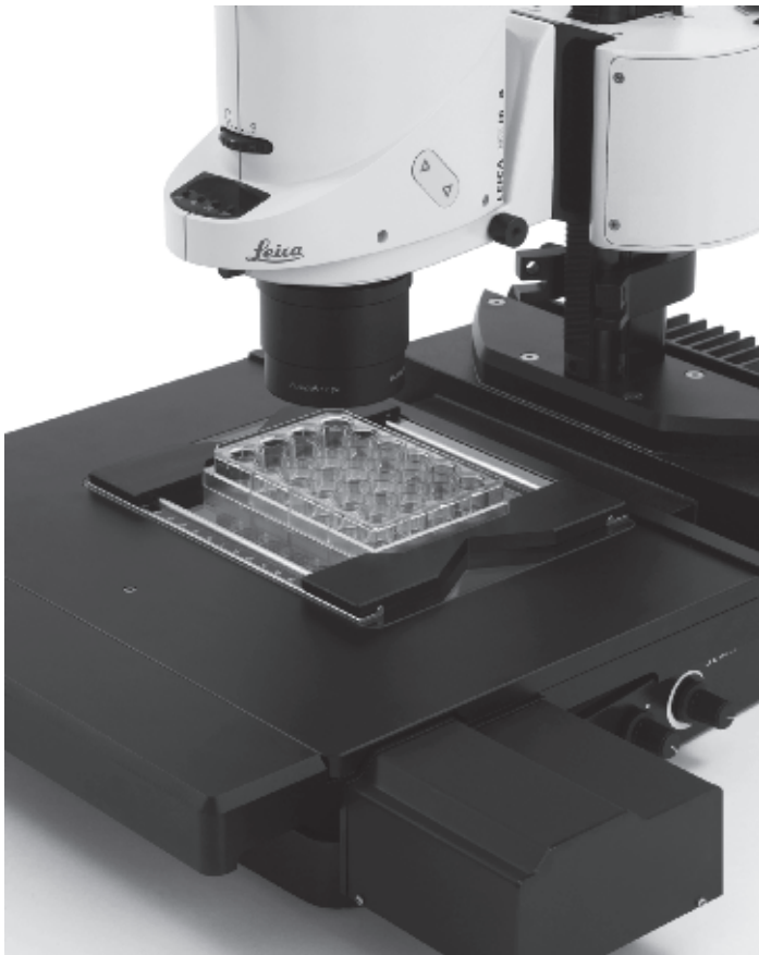
TL RCI™ transmitted light stand (10 446 352) With automated cross-stage Leica IsoPro™ (10 447 305)
