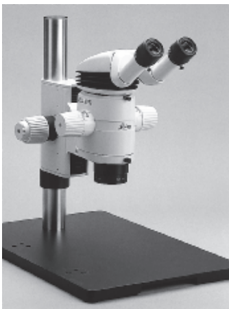
Drive housing with coarse/fine drive, Order no. 10 447 082, on the universal stand
