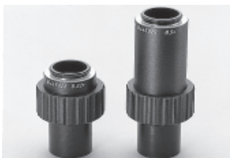
Video objectives with C-mount for CCD cameras: 0.32× for 1/3" and 0.5× for 1/2", additional video objectives: 0.63× and 0.8×
