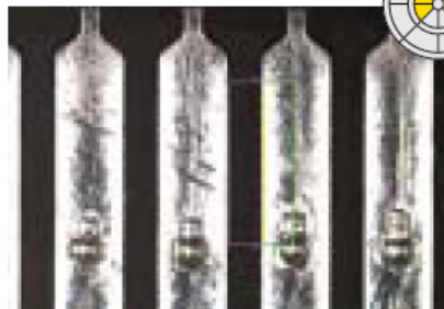
LED ring illumination (medium angles of incidence)
