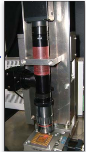
Navitar Ultra Precise Eye inspecting PCB components.
