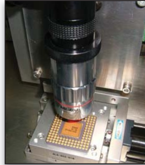
Navitar Ultra Precise Eye inspecting PCB components.
