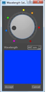
2) Change Emission wavelength by click on the Color selector the "Wavelengths Selector" will be opened and you can enter the exact emission wavelengths in "nm" for the filter set / fluorochromes.
