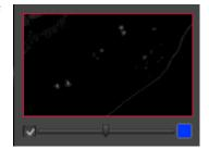
**Blue frame** rectangle indicates displaying of already recorded filter set image. The recorded image is activated and displayed on the image main window of GRYPHAX software. The image parameter of Fluorescence tool are deactivated.
