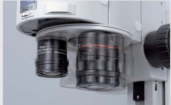
Three objective lenses can be simultaneously mounted to provide large zooming ratio.
