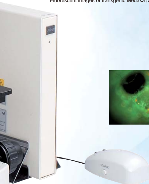
AZ100M combined with epi-fluorescence and diascope DIC accessories
