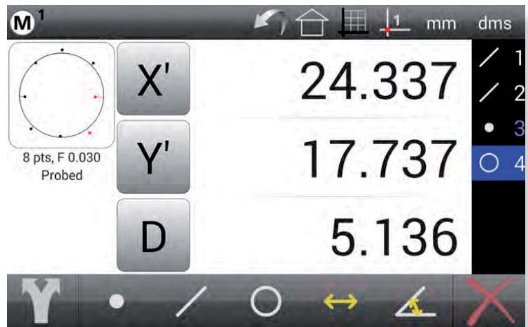
Feature detail views include position, dimension, points probed form error and a feature graphic
