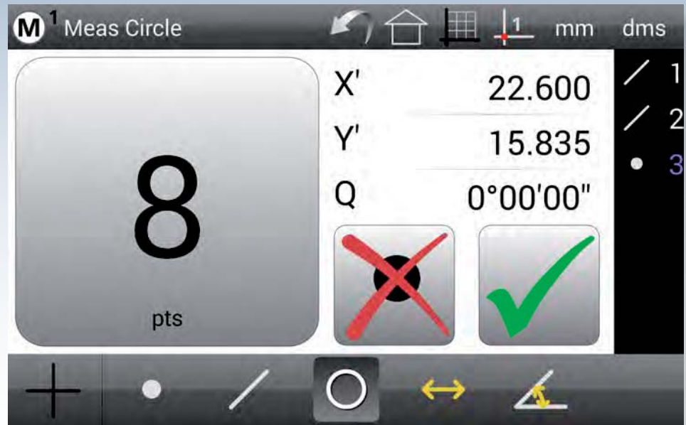
The M1 EdgeLogic™ function (optical edge detector systems only) enables gesture driven control of start and end measurement commands.
