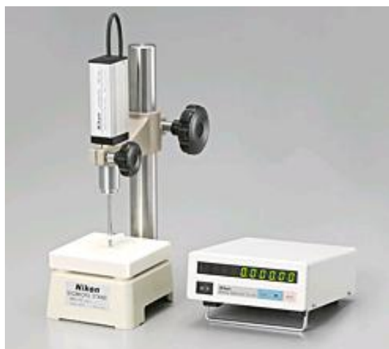
Left: standard ceramic stand for MF1001, shown with the counter (DRO) Nikon TC-101
