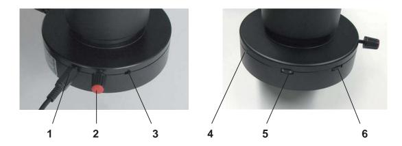
Attachment to the microscope objective, the power connection, on/off switching and brightness adjustment do not differ from the basic version. See the description in the above section entitled "Ringlight".
