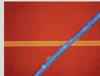
Epi-fluorescence observation of organic substance on wafer
