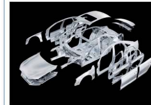
Body parts made of aluminum alloy
