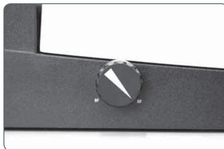
Button to toggle between bright field and dark field
