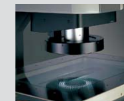
How the 8-sector LED ring illuminator works
