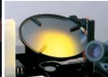
Back side center macro inspection (using a fiber optic illuminator)
