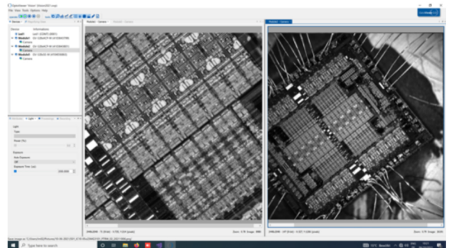
Fig. 15: The OptoViewer 2.0 allows simultaneous imaging of both cameras inside the linea XL module. Overview and 4x higher magnified details in full 5MP resolution due to the two separate optical paths.
