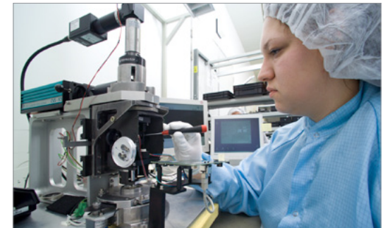
From around 7,000 reference points, the zoom body adjustment device calculates the zoom control curve.
