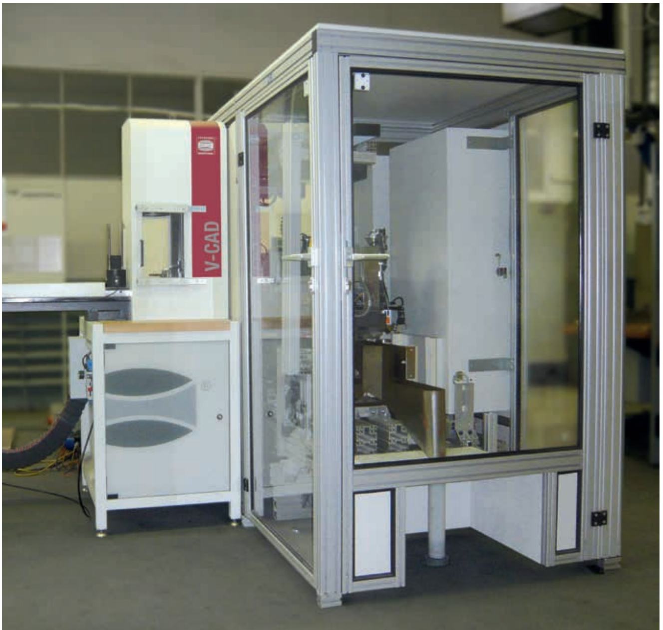
Measurement cell with two V-CAD modules and adjacent packaging unit
