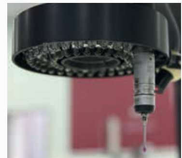
A valuable option for WM1 CNC: Touch-trigger probe TP200
