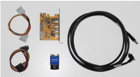
Power connector cables, PCIe interface card, camera, USB 3.0 cable
