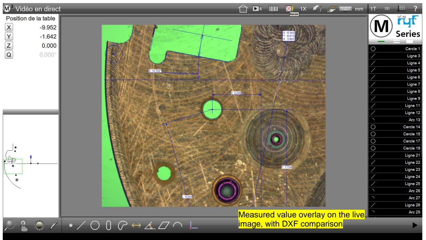
Live video: Optimum edge detection using "Measure Logic" or and active or fixed cross-hair
