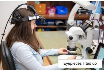
The two eyepieces in the headset may be controlled (up and down) with the foot pedal or by gestures.
