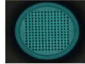
Mesh hole size = 0.07 x 0.07mm
